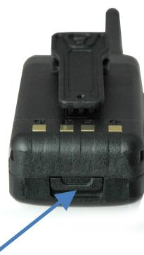
1. To uninstall the battery from the SC-1000 transceiver, **slide and hold the latch** on the bottom of the radio downwards. Then slide the battery pack backwards towards the latch to remove it.
