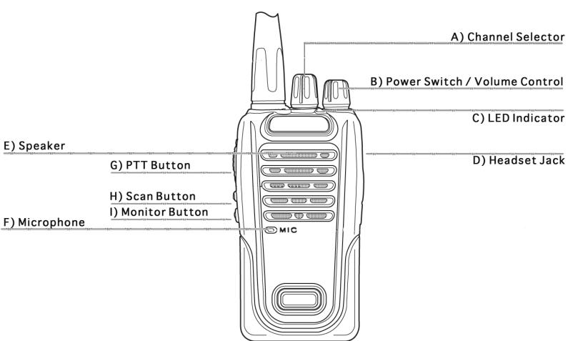
Each Scrambler Plus is factory programmed to provide discreet private two-way voice contact. All outgoing transmissions are digitally encrypted and scrambled to prevent eavesdropping. In addition, CTCSS frequency guard protects the receive circuit by blocking outside interference. Combined, these features ensure that communications remain completely private.
